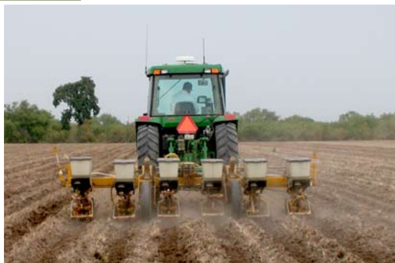
Figure 4. Buffalo ridge-tillage seeder planting cotton into barley cover crop residue, Borba Farms, Riverdale, California, May 14, 2003. Photo: J. P. Mitchell.
