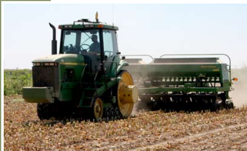
Figure 1. John Deere 1590 no-tillage drill seeding sorghum-sudan hybrid into corn stubble, Barcellos Farms, Tipton, California, July 24, 2005. Photo: J. P. Mitchell.
