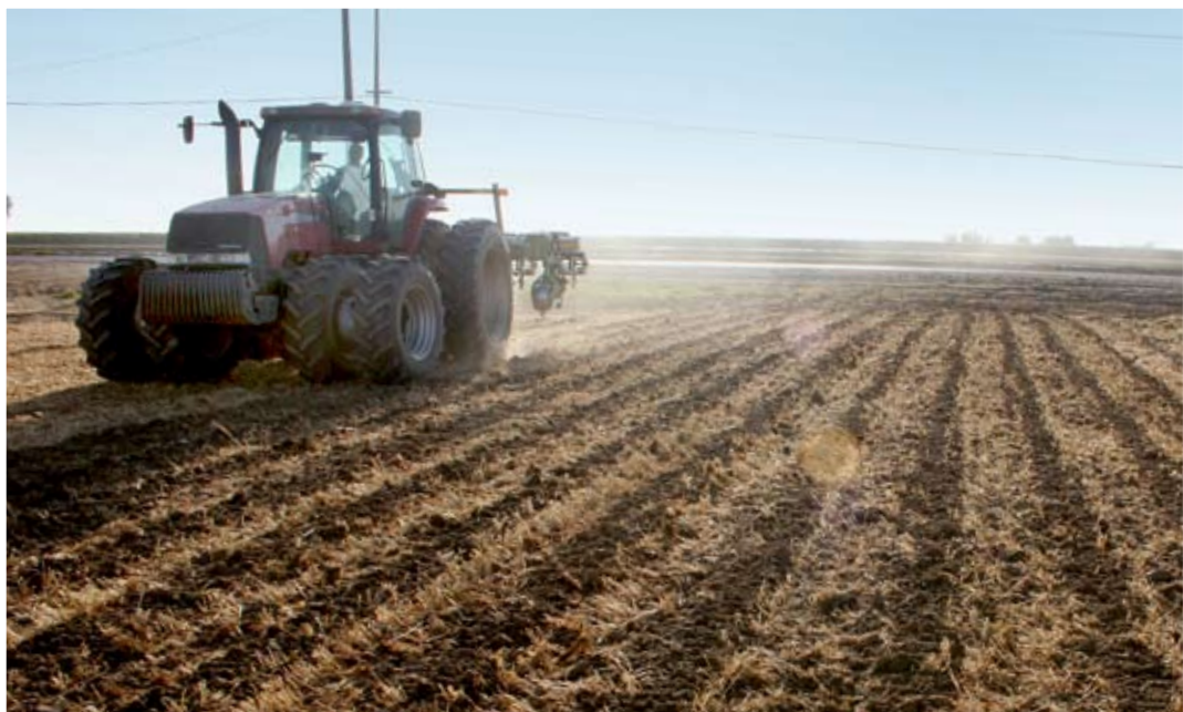
Figure 2. Orthman 1-tRIPr strip-tiller in wheat stubble prior to forage corn planting, Giacomazzi Dairy, Hanford, California, May 16, 2006. Photo: J. P. Mitchell.
