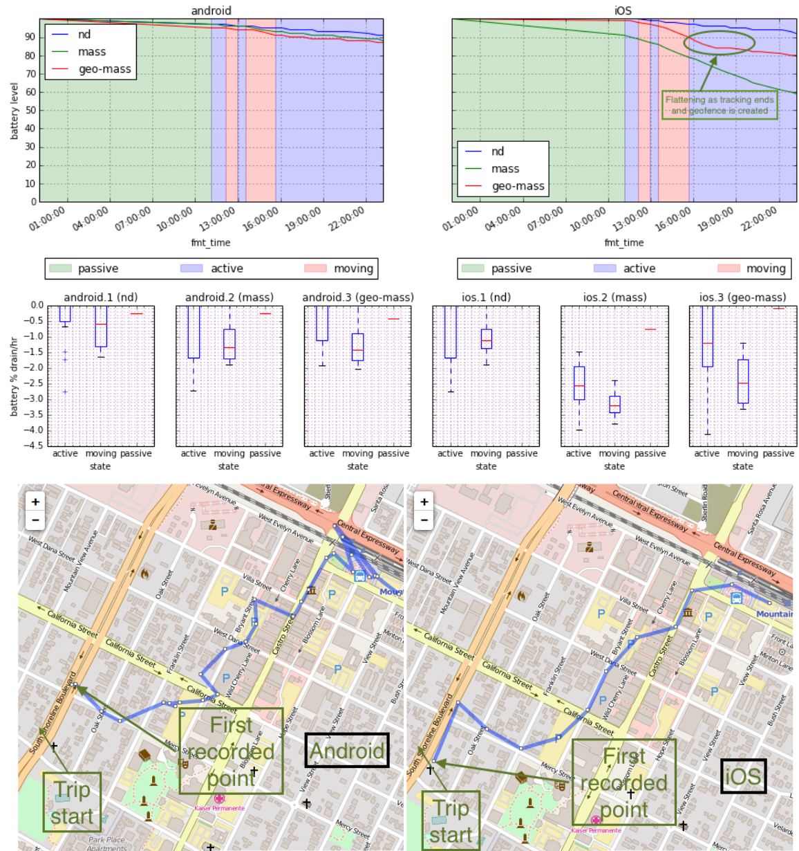
Figure 4.4. Evaluation of geofencing while collecting data with medium accuracy, and a slow sampling rate. Regimes are no data collection (nd), medium accuracy fast sampling (mass) and geofenced medium accuracy fast sampling (geo-mass). The top graph shows the change in battery level over 24 hours. The middle graph shows the rate of drain in %/hr in the active, moving and passive states. The bottom map shows the extent of the error on each platform at the beginning of the trip.
