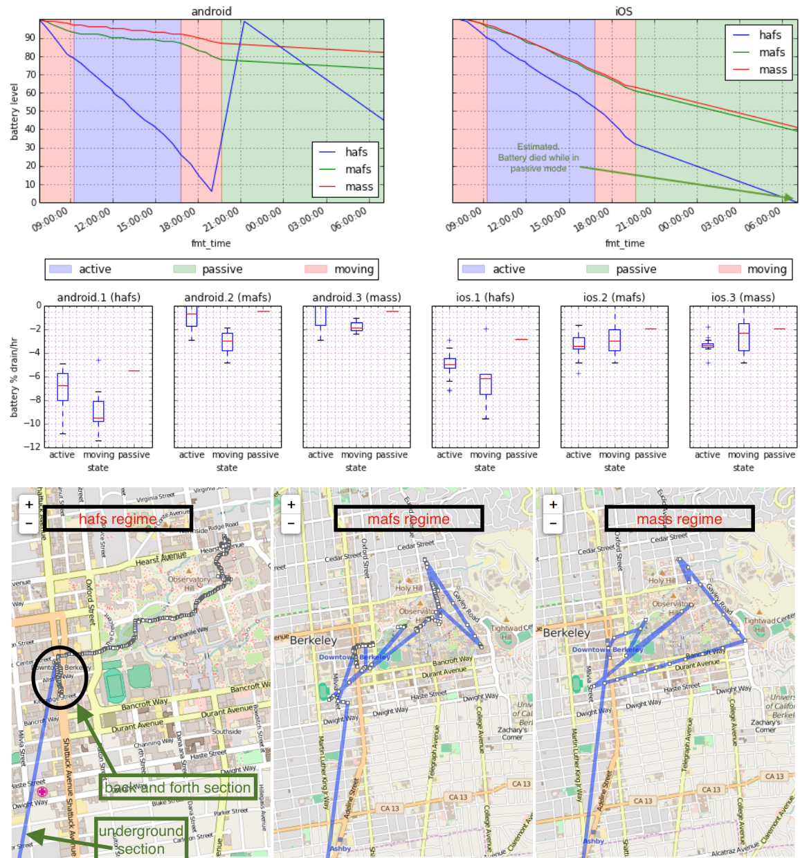
Figure 4.1. Comparison of three existing data collection regimes with no geofencing. Regimes are high accuracy fast sampling ( hafs ), medium accuracy fast sampling ( mafs ) and medium accuracy slow sampling ( mass ). The top graph shows the change in battery level over 24 hours. The middle graph shows the rate of drain in %/hr in the three states. The bottom map shows the data points collected by each regime and provides an intuition of what the different accuracy levels correspond to.
