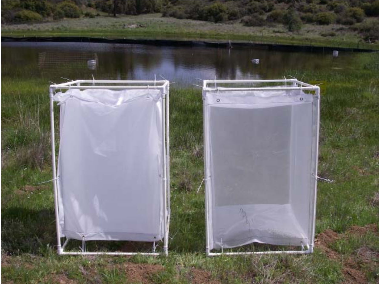
Figure 2.2. Example of 0.5 m x 0.5 m x 1 m 35µm “fine” mesh cage that is parasite impermeable (left) and 500µm “coarse” mesh that is parasite permeable (right).
