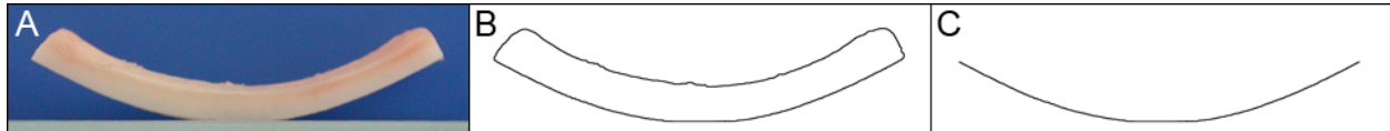
Figure 2. Converting the cartilage slice into a single curve. A) The original photograph is opened in Photoshop. B) The outline is automatically traced using the magic wand tool. C) The eraser tool is used so that only the curve on the convex side of the specimen remains.
