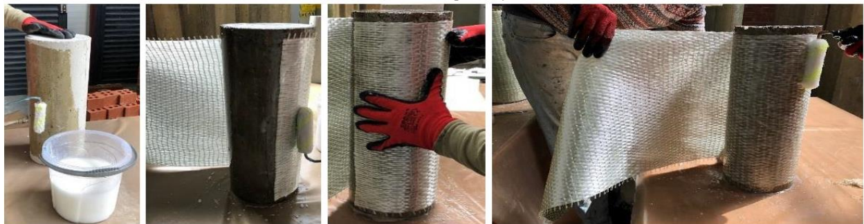
(b) GFRP Composite System
