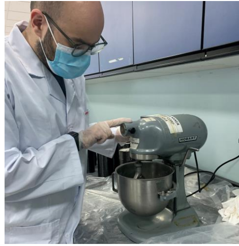
b) Mixing of epoxy matrix
