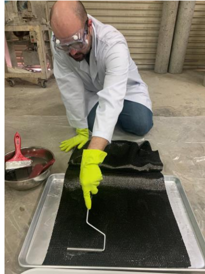
c) Impregnating the carbon fiber sheet with the epoxy matrix
