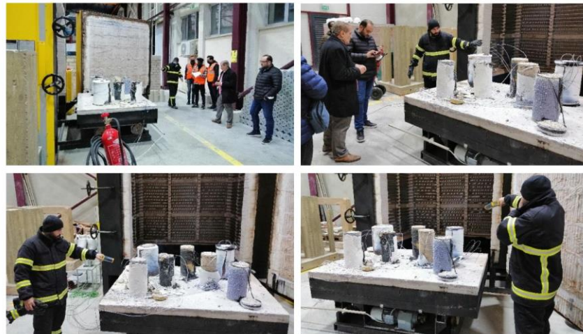
Figure 4-7: Opening the furnace door and first measurements of surface temperature after Test-2
