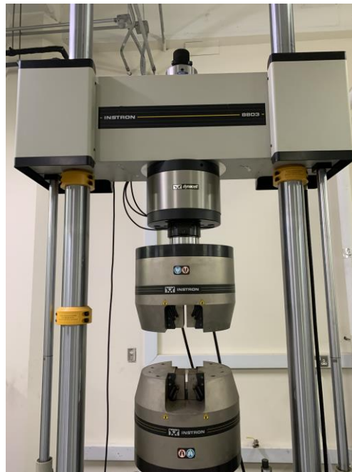
Figure 6-5: Instron Machine used for Tensile Test
