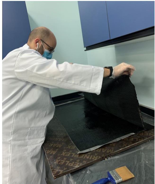
d) Laminating second ply of CFRP laminate
