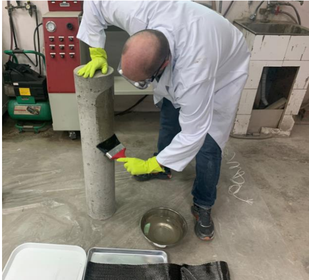
c) Applying a primer epoxy coating on the concrete specimens
