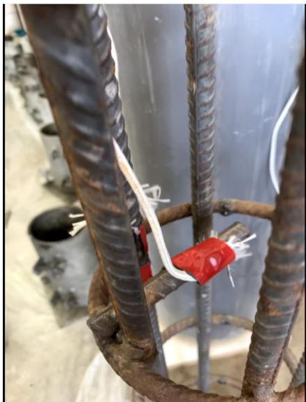
a) Thermocouple location in the center of the column
