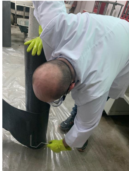
d) Rolling the carbon fiber fabric on the column specimen (bottom half)
