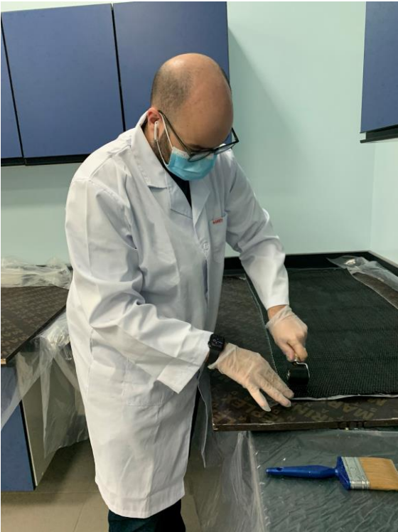
c) Rolling first ply of the CFRP laminate
