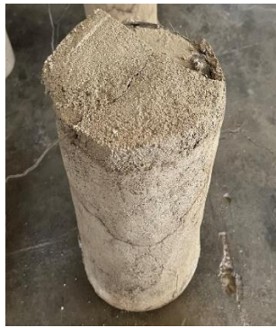
a) View of fire protected specimen after cooling
