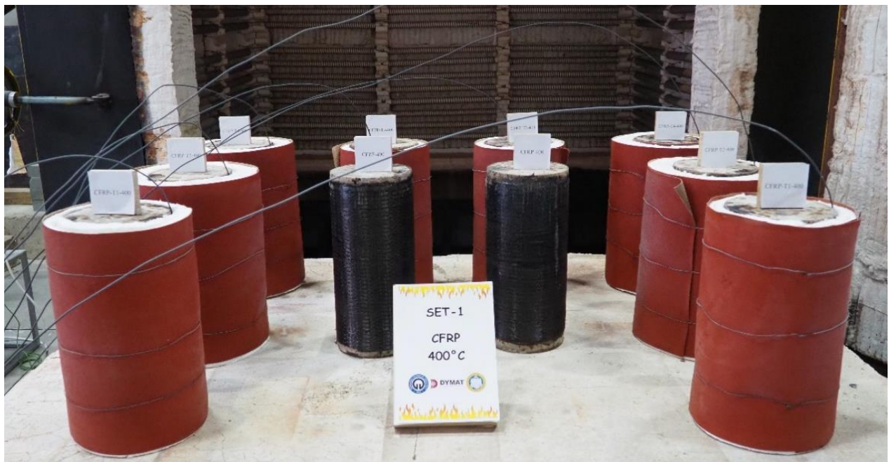
Figure 3-9: View of CFRP System-A specimens after exposure to Thermal Protocol-2 (400°C)
