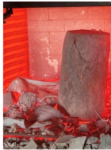
d) Inside view of the furnace post-thermal exposure 700°C
