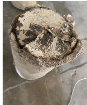
b) View of fire protected specimen with the top removed
