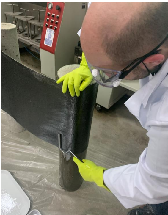
d) Rolling the carbon fiber fabric on the column specimen (top half)
