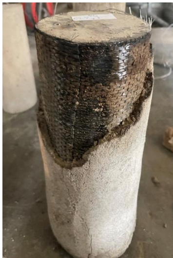
c) View of FRP surface after thermal exposure
