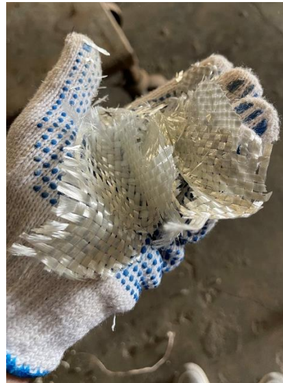
g) Fire protected (1 layer) GFRP post-exposure to 700°C
