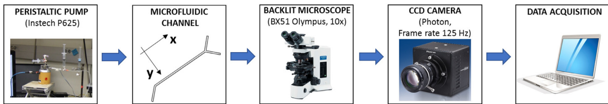
Fig. 1. Experimental setup scheme. The RBCs sample was pumped in the micro-channel by a peristaltic pump (Instech P625). The process was monitored optically by using a backlit white light microscope (BX51, Olympus), with a magnification of 10X and coupled with a high-speed CCD (PCA 1024, Photron).
