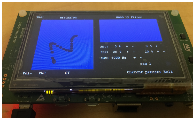
Figure 3.11 - Resonating filter bank on an STM32F7 board
