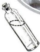
In circle, camera that makes records of film showing the inclination of well being dug. Right, whipstock that is set at bottom of well to deflect bit. Left, acid-etched bottle that shows slant of the well
