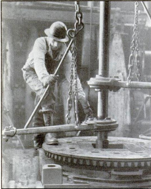
The large-toothed circle in the photo above is the rotary table that grips the drill pipe and imparts a turning motion to the bit. By tilting this table, the well can be deflected right from the start
