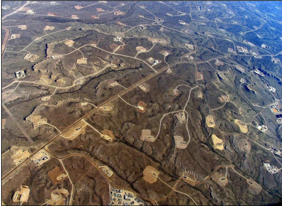
Figure 24: Pad Drilling with Hydraulic Fracturing in Upper Green River Valley, Wyoming.
