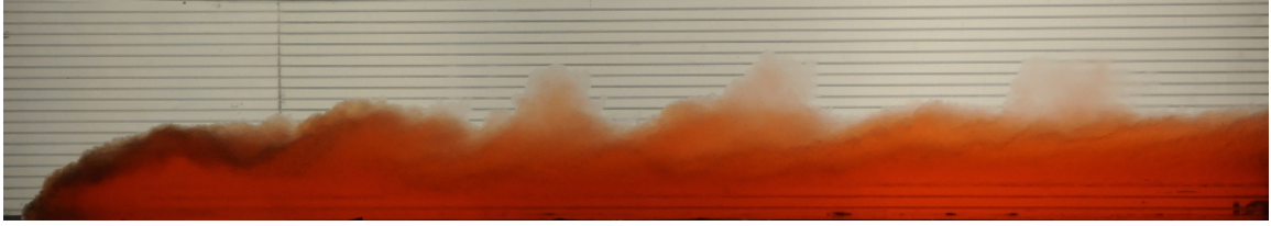
Figure 2: Visualization of the gravity current with Re = 72,000 (Experiment 6; table 1). The current is dyed with food colouring and viewed against a translucent lined sheet.
