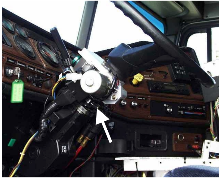
Fig. 4 Steering actuator mounted on the steering column
