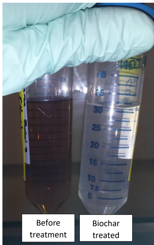
Figure 11. Biochar-treated food waste permeate (FWP) before and after treatment with 1 g of walnut-derived biochar per 40 mL FWP. Photo credit: Tyler Barzee.
