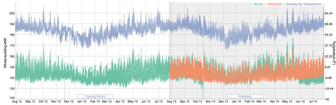
Figure 1. Actual and model-predicted energy data, overlaid with outside air temperature, for a 12-month pre-installation period (training period) and 12-month post-installation period (prediction period).
