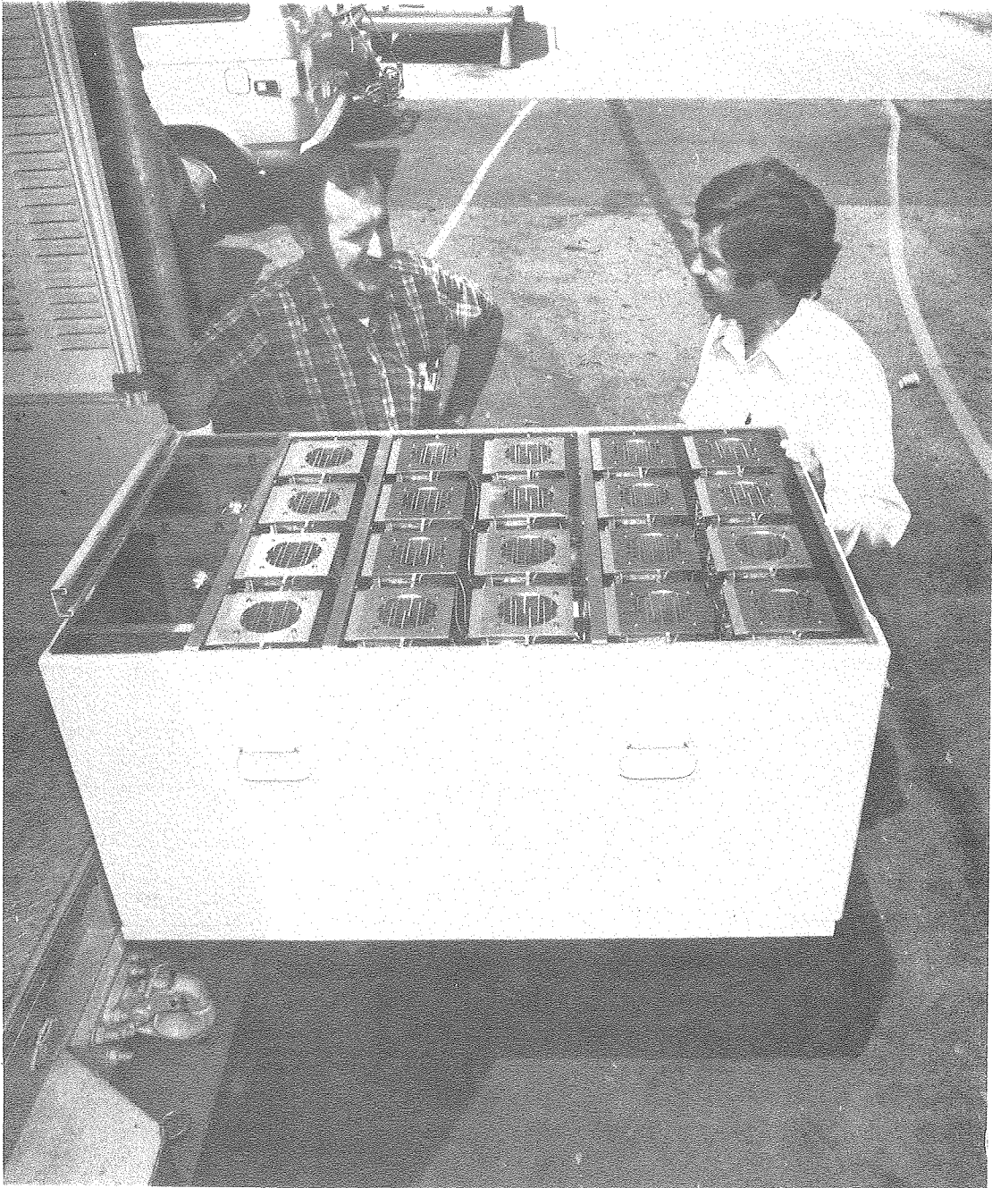
Figure 3. The crate with its cover removed, showing the modular arrays of transistor switches and the full-wave rectifier at left.
