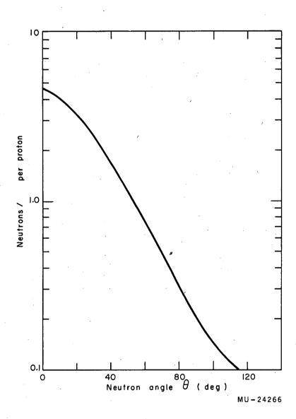
Fig. 2. Angular distribution of neutrons, over 150 Mev in energy, from 1 mfp of Cu traversed by 6.3-Bev protons.
