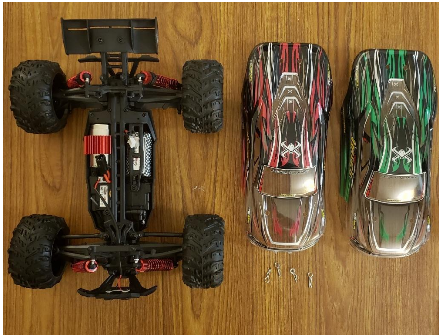
Figure 1. Internal view of the MIEBELY model RC car shows a removable car body, allowing for simple access to vital electric components.
