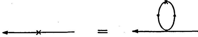
Fig.6. The gap equation for the t -quark mass. The cross denotes m_t .
