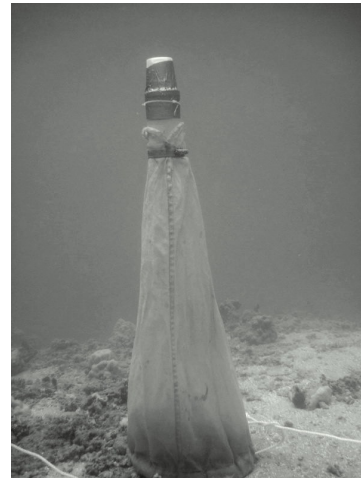
Figure 2. An example of an emergence trap over substrate.
