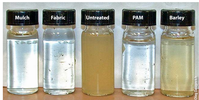
FIG. 2. Turbidity of runoff water in first flush of runoff from raspberry post rows with different treatments and untreated bare soil at Somis on March 10, 2018.
