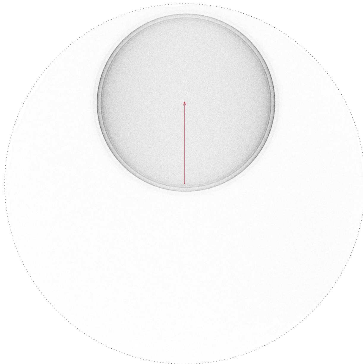
Figure 5.12: Velocity-map image of photoelectrons detached at 733 nm (1.69 eV) from O accelerated to 5 keV. The detector area is outlined by the dotted circle. The red arrow shows the image displacement due to the drift velocity inherited by the electrons from the fast parent ions.
