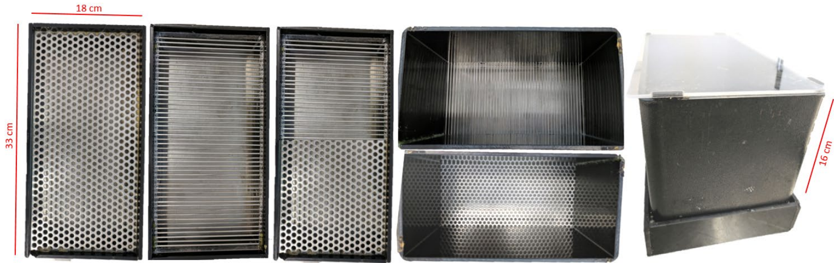
Appendix C Figure 1. Conditioned place preference (CPP) chambers used in all experiments. Chambers are same from Zombeck (2008). The interchangeable stainless-steel bottoms have holes or a grid of rods for conditioning, or a combination of hole/grid for preference testing. The walls are black, and the lids are clear plexiglass to allow for videotaping from above.
