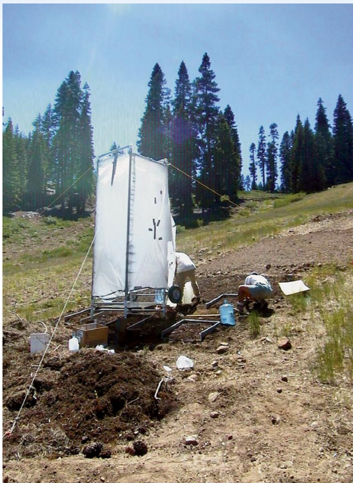
A rainfall simulator was used to measure sediments in runoff under a variety of soil and groundcover conditions in the Lake Tahoe Basin.
