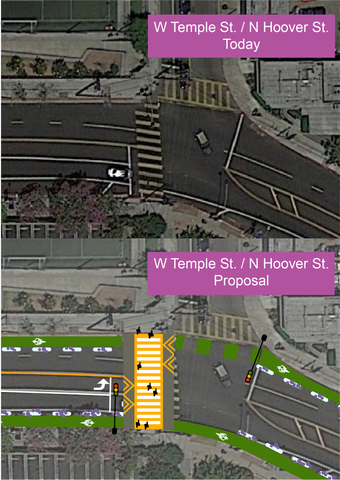
Design by Erika Kulpa & Jorge Cáñez, May 2020 Here I propose a raised crossing, a new signal, and the protected bikeways
