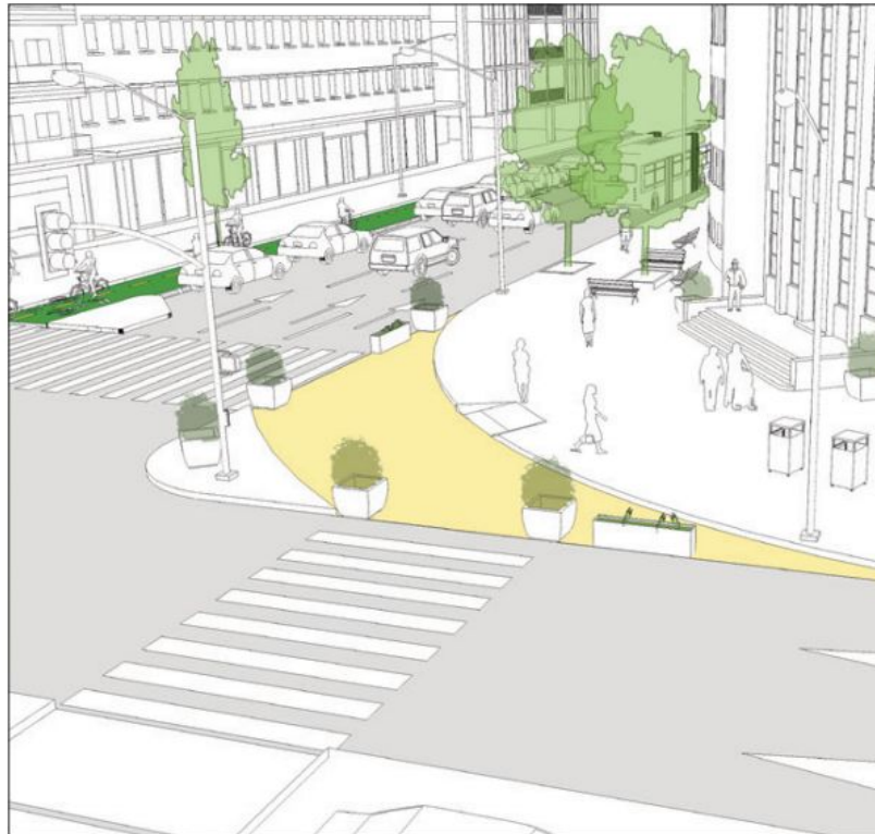
Figure 35. Slip lane removal
