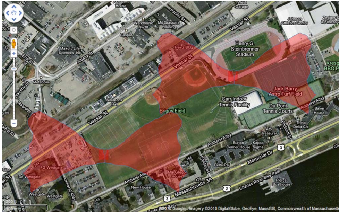
Figure 36: Expected topography of shadow flicker effect over the west side of MIT campus for two particular wind turbine sites
