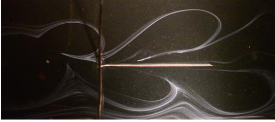
Fig. 3. Image of the flow near the flexible plate. The cylinder which generates the vortices is barely visible on the left-hand side of the picture. The vertical wire constrains the axis of the plate's leading edge.
