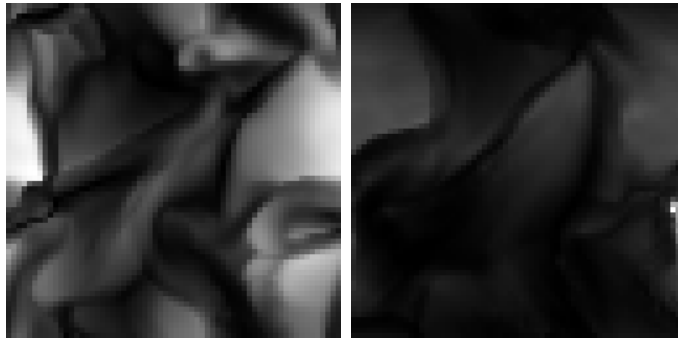
Figure 3.13: A demonstration of an instability that is believed to be caused by improper reconstruction of the electric field in an unsplit method. Both panels show density in driven turbulence at Mach 3. The left panel has no magnetic field, the panel at right has B = [0, 0, \sqrt{2}] . The spike in the right is an unavoidable explosion.
