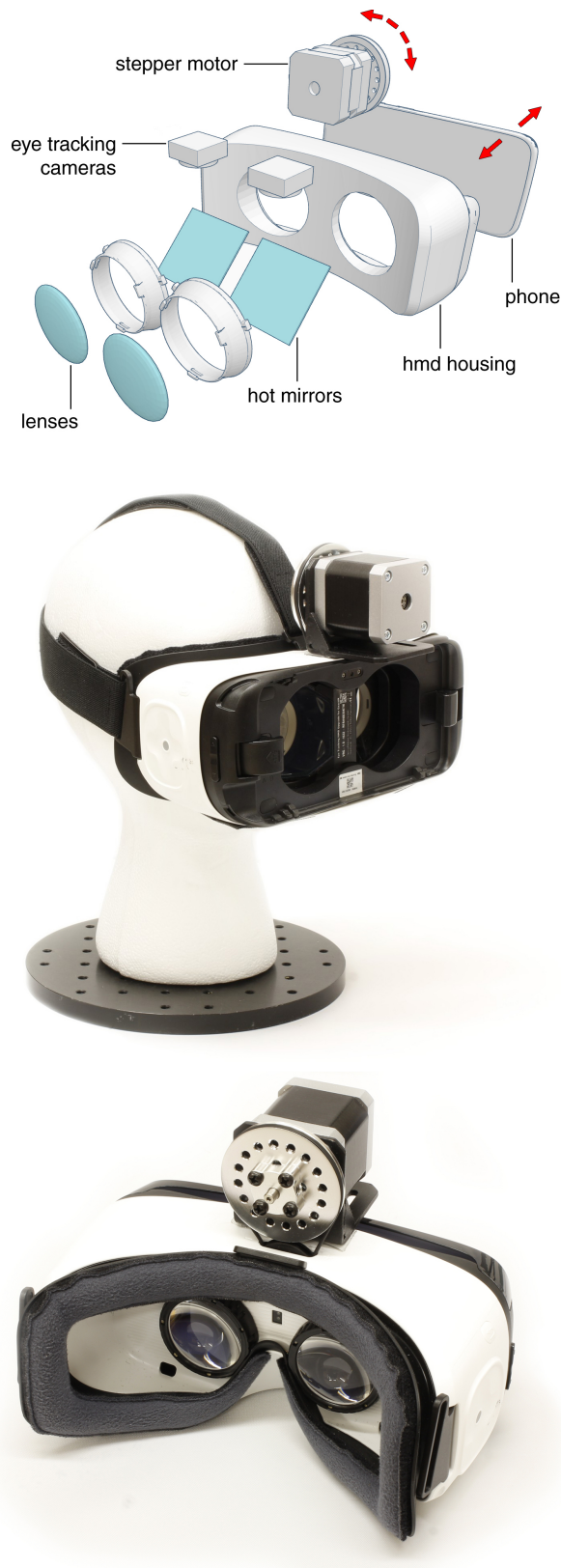
Fig. S2. A conventional near-eye display (Samsung Gear VR) is augmented by a gaze tracker and a motor that is capable of adjusting the physical distance between screen and lenses.
