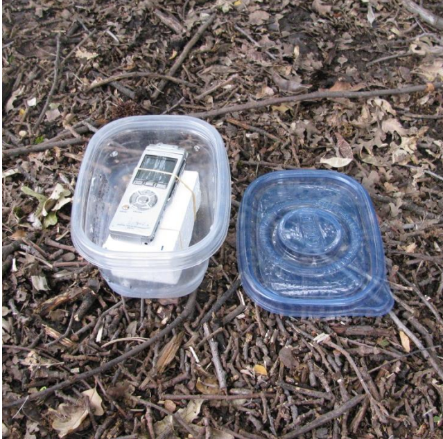
Figure S1. An automated recorder (Olympus DS-40 digital voice recorder, www.olympusamerica.com ) and its protective container used for surveying common forest birds in northern California. Each device was programmed to automatically record sounds during 5-minute survey periods at 3 times each morning repeated over 3 consecutive days.
