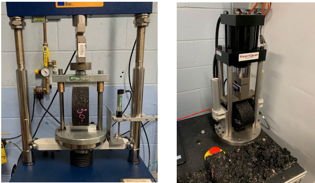
Figure 2.6: Testing machine for IDEAL cracking test with a specimen.
