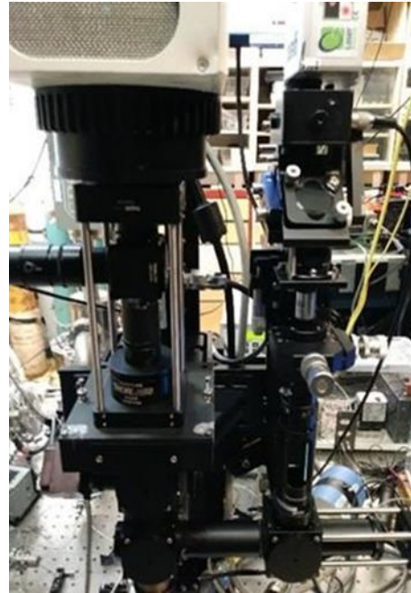
Figure 7 Picture of the optics setup along with direct mounted laser assembly, 3 axis spatial filter assembly, CCD sensor, 200mm Nikon tube lens, and filter wheel assembly are shown
