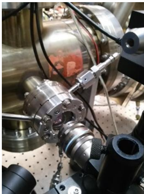
Figure 2 Viewport, part of chamber with sample holder area, microscope objective
