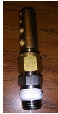
Figure 5 Sample holder assembly with \frac{1}{4} inch outer diameter (OD), 240V, 300W Watlow cartridge heater. The sample holder is made of gold plated \frac{1}{2} inch OD molybdenum covering this heater assembly. \frac{1}{4} Swagelok fitting seals gas tight connection to the \frac{1}{4} NPT thread which seals chamber and ambient.
