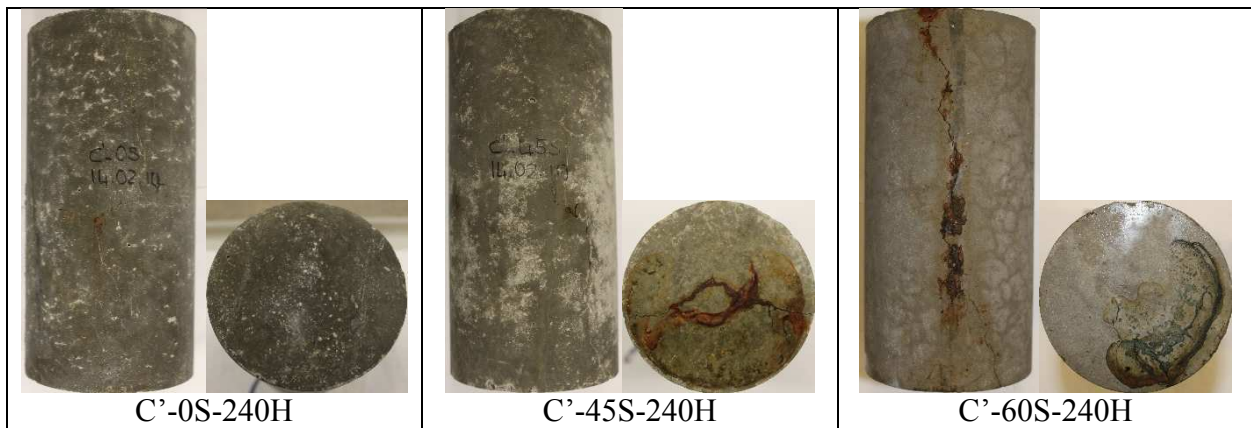
Figure 5.10: Corrosion-induced cracks for plain concrete with slow applied current
