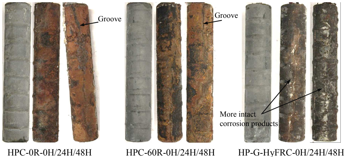
Figure 3.15: Bar surfaces showing no corrosion for samples with no applied current and uniform corrosion for samples with 24 and 48 hours of applied current
