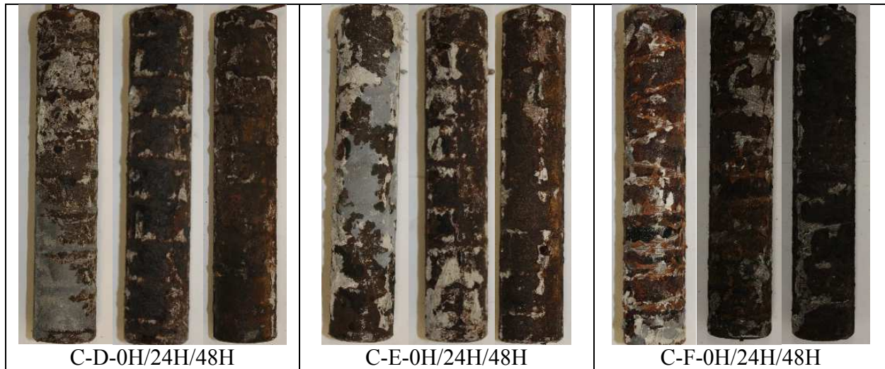
Figure 6.12: Corrosion on bar surfaces showing patches of corrosion on C-D-0H/C-E-0H and uniform corrosion for all other samples
