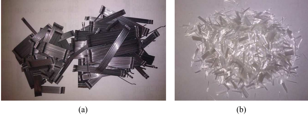
Figure 5.1: Fibers used in the study: (a) 30 mm and 60 mm hooked-end steel fibers, and (b) PVA microfibers
