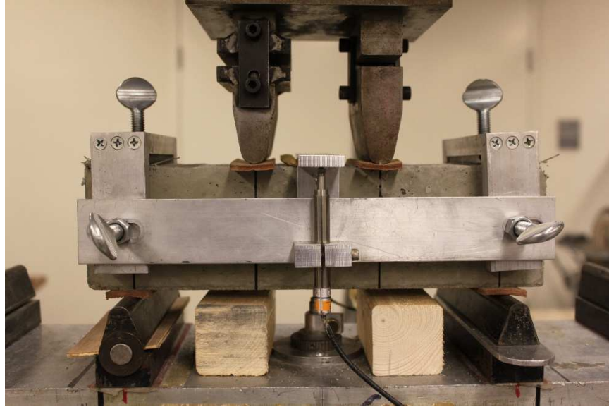
Figure 2.2: Flexural test setup
