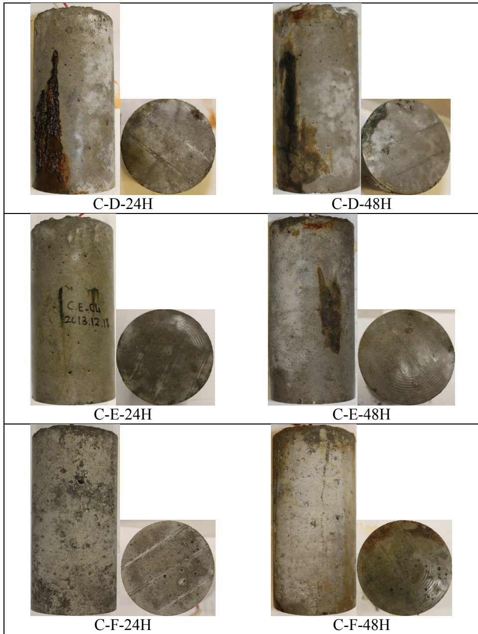
Figure 6.9: Cracking on surfaces of samples with different regimes of applied current
