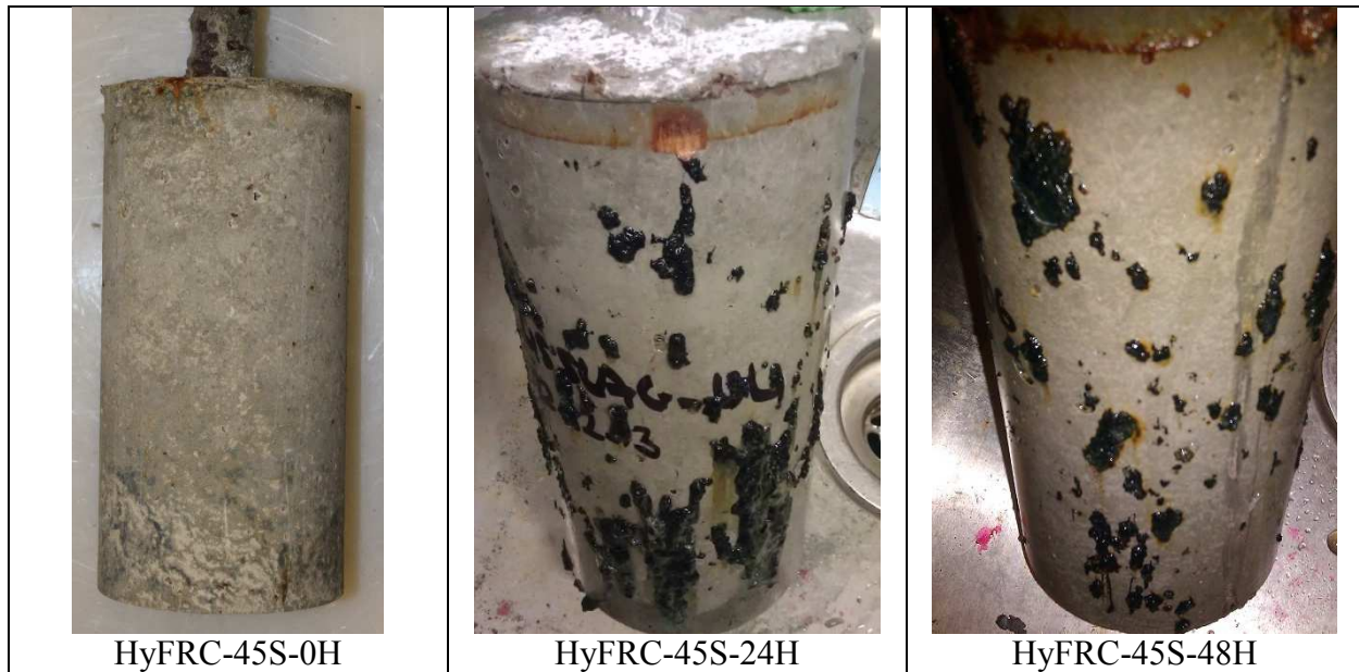
Figure 5.13: Fiber corrosion on surfaces of HyFRC-45S
