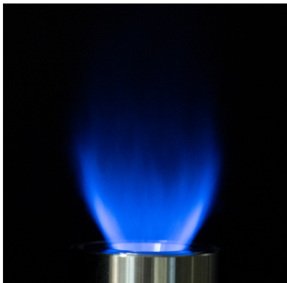
Figure 4.4: GENSETS 14 mm LSB fired in the open with a 30-degree quarl at \phi = 0.75 showing a highly stable, diverging flow field.
