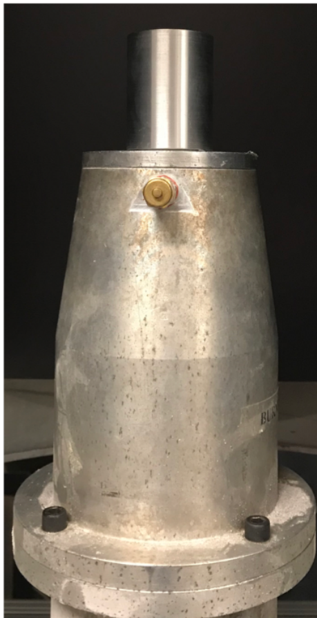
Figure 3.4: Contoured wall plenum with 1" swirler mount shown on top in lighter stainless steel material.
