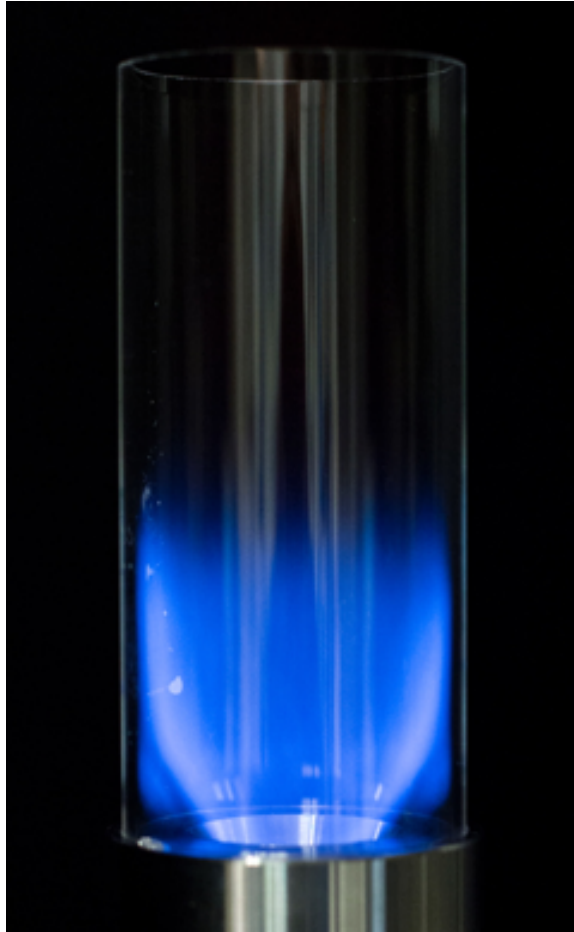
Figure 4.5: 14 mm GENSETS LSB with quarl and quartz enclosure at \phi = 0.75 showing a highly stable and short flame.
