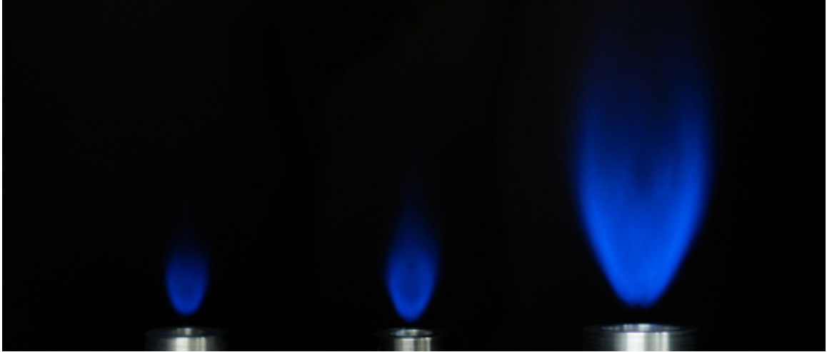
Figure 4.12: Images of 12 mm, 14 mm, 25.4 mm (from left to right) LSB Operating with U_0 = 10 m/s, \phi = 0.80 .
