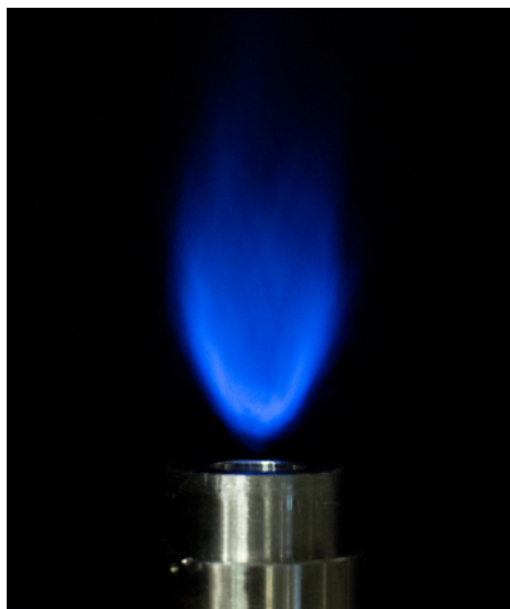
Figure 4.1: GENSETS LSB fired in the open air (no enclosure or quarl) at \phi = 0.75 showing a highly-stable, short, bowl-shaped flame.
