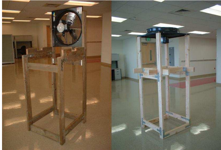
Figure 4.10: Absorber/IHX and Regenerator stands
