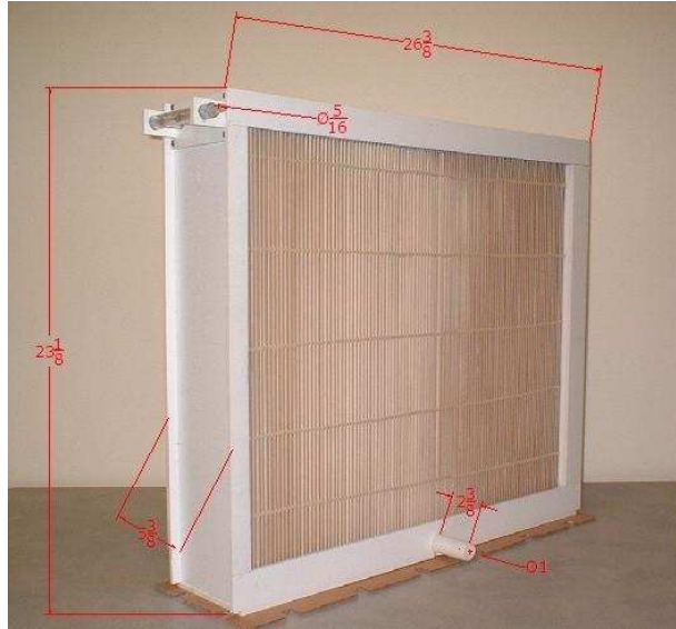
Figure 4.6: Absorber by AIL Research. 100 plates, 0.4m^3/s (833 cfm), 1.1^\circ C ( 34^\circ F ) dry-bulb and 0^\circ C ( 32^\circ F ) dew point. Figure shows the dimensions in British units because of design.
