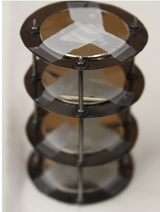
Figure 5.10: Tungsten rods used to hold the four foil stacks in the empty HTOAD configuration.
