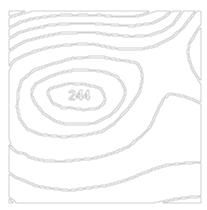
contour line structure. This system is based on storing a vector version of the traditional printed contour line. This model is convenient because minimal hardware and software is required to transform hard-copy map contour lines into digital contour lines. However, algorithm development is very difficult and of the three models this one requires the most storage space.
