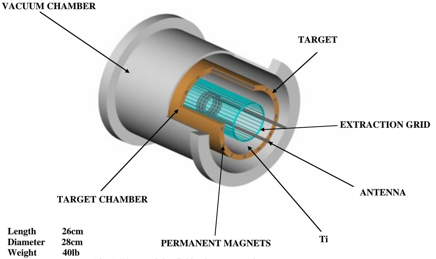
Fig. 1 The coaxial radial ion beam extraction neutron generator.
