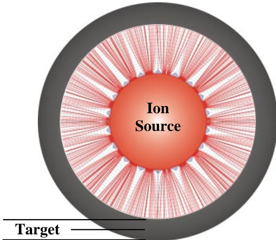
Fig. 2 Cross-sectional view of the coaxial neutron generator with ion beam trajectories computed by using the IGUN simulation code.
