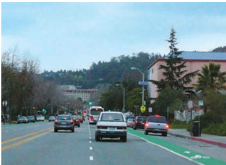
Figure 12. Commercial Street – Green Painted Bicycle Lane next to Parking Lane
