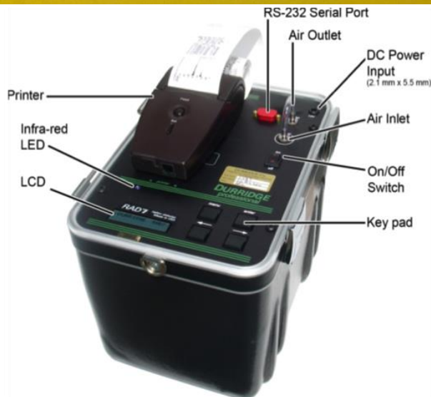
Figure 6: RAD7 device setup in conjunction with the membrane contactor and desiccant tube to ensure no water vapor enters into the RAD7 sensor chamber. (A) Setup developed by Schmidt et al. (2008) and (B) example of RAD7 device controls and air inlet / outlet.
