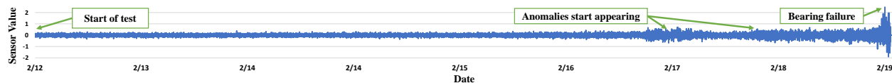
Figure 3.2: Accelerometer Data from Test 2 of the NASA Dataset [1]. Symptoms of bearing failure can be seen on 2/17 and 2/18 before the bearing’s outer race failed on 2/19.
