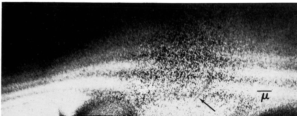
Figure 2. Intense knock-on radiation damage in Cu-14 at. % Al alloy after 1 hr exposure at 1 MeV (observations from 1 MeV instrument, Nagoya University, Japan); the stacking fault arrowed is barely visible.
