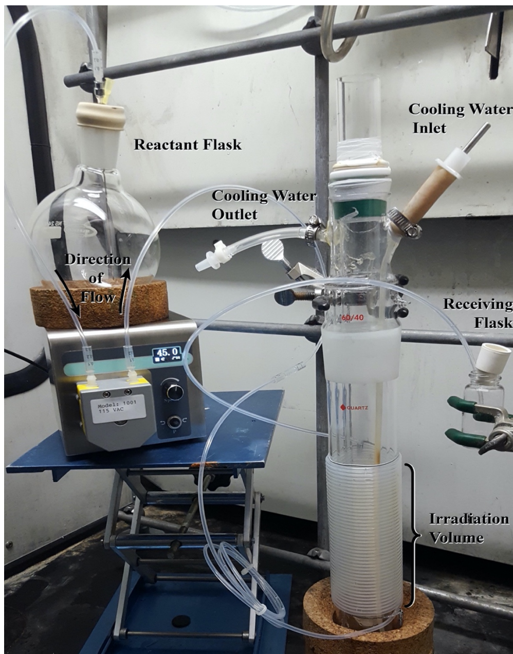
Figure 1.4.1 Flow Reactor Setup. Arrows indicate direction of flow.
