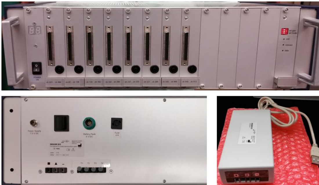
Figure 6.5. Top: front panel of 512-channel neuroConn DIGGER data acquisition system. Each module has a 68-pin SCSI connector and a banana plug for connecting reference signals of different modules together. Voltage range and gain are set with small DIP switch near upper right corner. Bottom left: rear panel of DIGGER system showing connections for outlet power, battery power, and fiber optic outputs. Bottom right: optical POF signal to USB converter.
