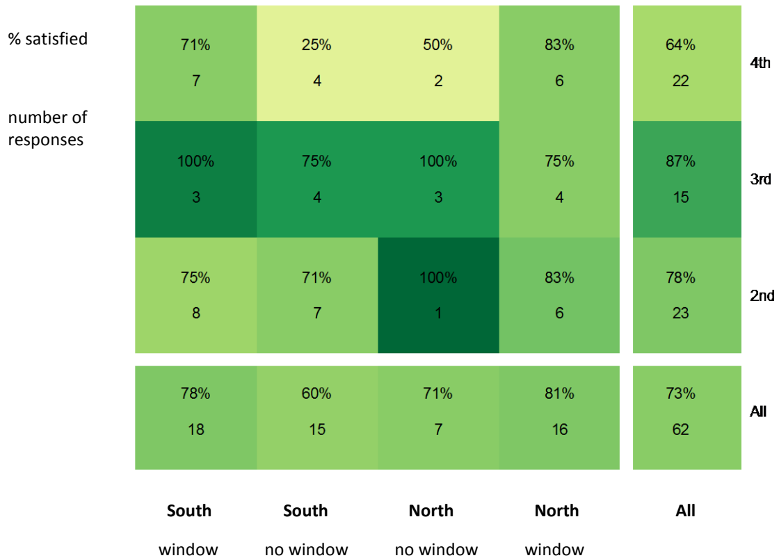
Figure 10. Air quality satisfaction by floor and orientation.
