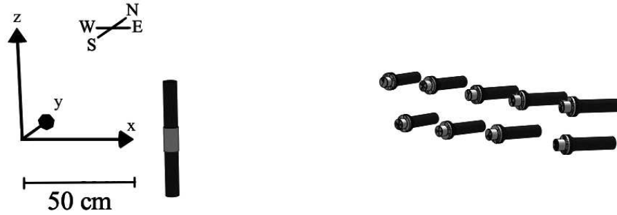
Figure 3: Schematic of the detector array configuration for the EJ-276 proton light yield measurement. The neutron beam traveled along the x -axis through the target scintillator with dual-ended readout with observation detectors positioned at forward angles with respect to the incoming beam. Similar configurations were used for the EJ-309 and organic glass proton light yield measurements.
