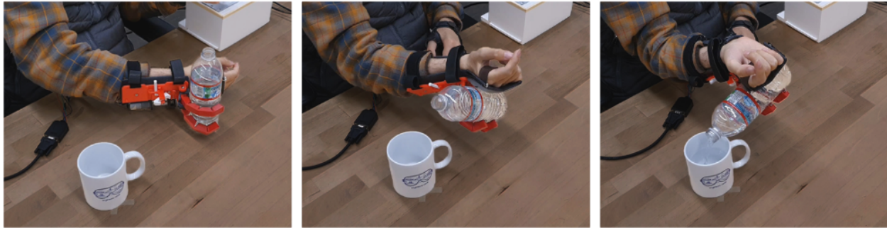
Figure 4.13: The subject with SCI picks up a water-bottle and pours water into a mug without spilling.
