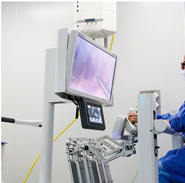
Fig. 19 Rob Surgical Systems—S Bitrack System Surgeon Console
