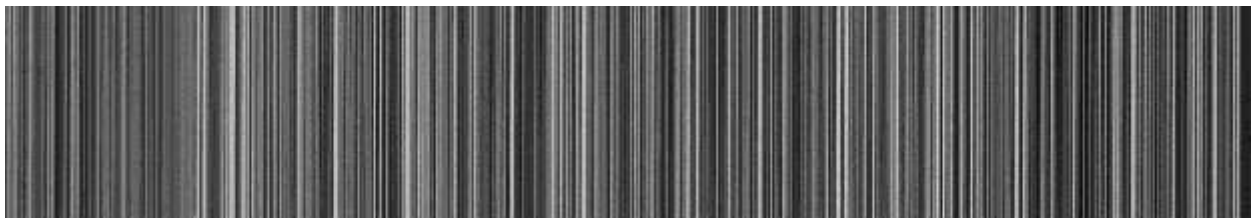
FIG. 6. TEM image of a cross section of the BPRML sample obtained by analytically stitching the eight images measured at the electron energy of 17.5 keV. The left-hand side of the image corresponds to the top of the sample in Fig. 5.
