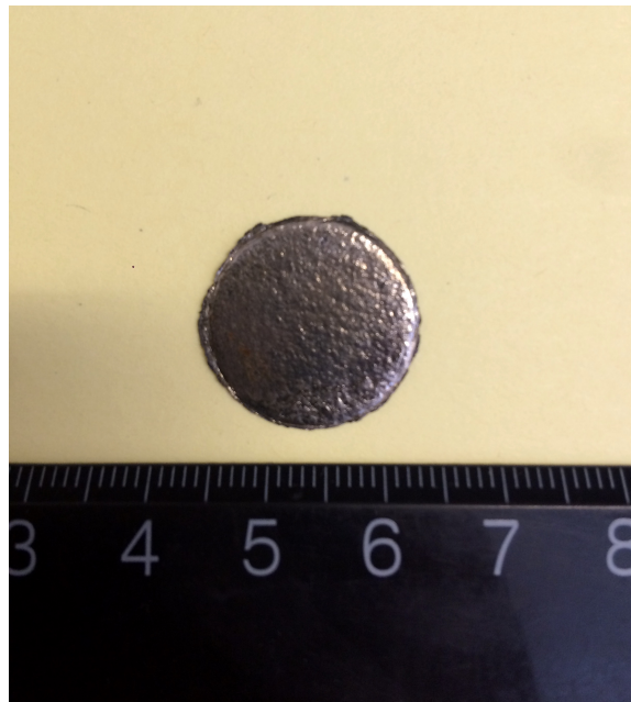
Figure 13: SPS sample after removing the graphite residual.
