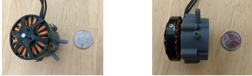
Figure 4.46: Mini high pressure regenerative turbine pump for small robotic system liquid cooling purposes.
