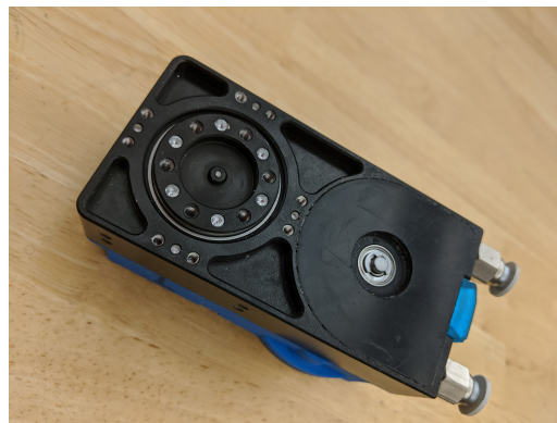
Figure 4.4: Koala BEAR actuator module.
