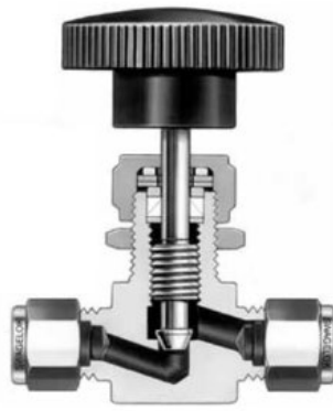
SS-1KS4 – V needle valve 4.4 mm orifice (fully open) C_v = 0.37
