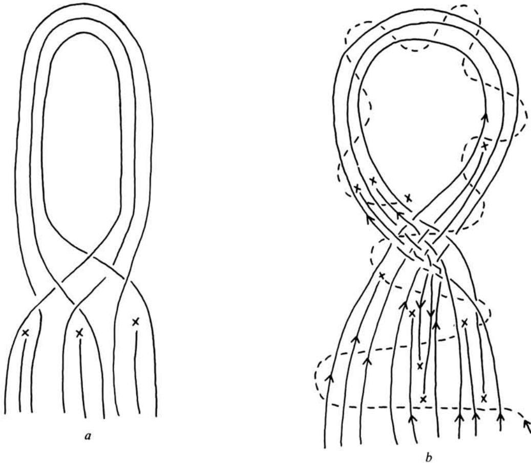
Fig. 3. Schematic view of splicing of the elements to form the long loop and the eye; *a*, long loop made on fold of three 2-ply twines and the supplemental twines inserted to augment the diameter of the main rope; *b*, eye with the ending of each of the 2-ply twine elements. *x* indicates the end of each element. The fine sewing twine terminates at the base of the eye.
